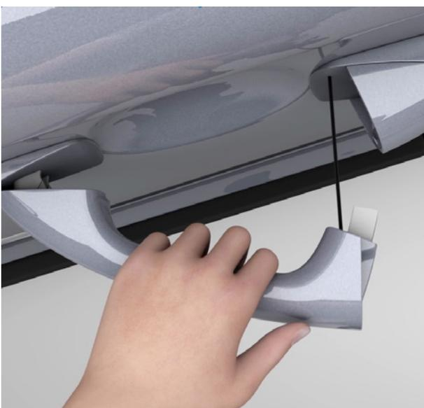
Mechanical crash redundancy still requires a rudimentary external activation chain, however, this can be designed much easier — adapted to the exceptional situation of an accident. For example, inside and outside, it suffices to have handles arranged behind trim strips in conjunction with simple, lever-optimized pullers.
