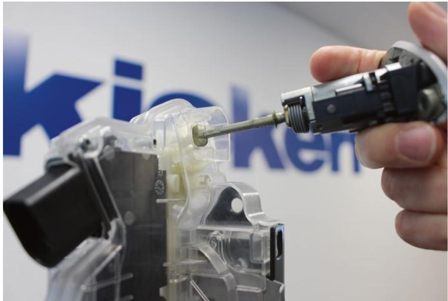
**FIGURE 1** The mechanical connection between lock cylinder and latch demands their physical proximity (© Kiekert)
