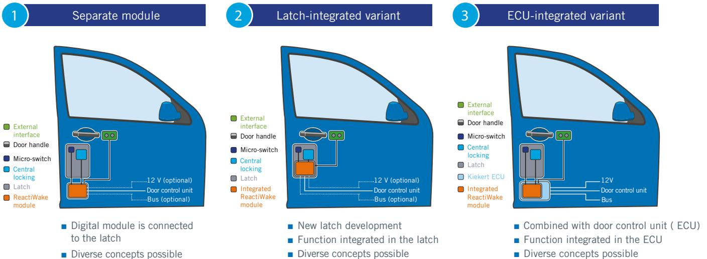
FIGURE 5 Three examples of system architecture: separate module, latch-integrated and ECU-integrated variant (© Kiekert)
